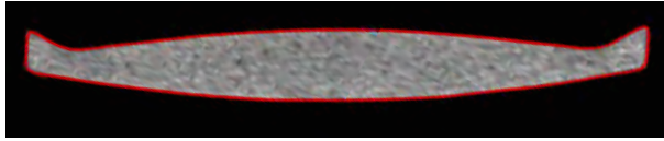
Supplementary Figure 8.1: \mu CT scan of the ZCB00. The images were acquired on a SkyScan 1076 \mu CT scanner (Bruker Corporation) using a round scanning trajectory with a step size of 0.3 degrees, an exposure of 1250 ms and an isotropic resolution of 9 \mu m. The 3D images were automatically segmented using an in-house developed analysis pipeline in MeVisLab (version 3.0.2, MeVis Medical Solutions AG), and the result is shown in red.
